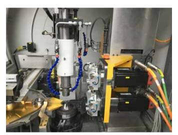
Outer ring outside diameter 85 - 200 mm Inner ring inner diameter 50 – 180 mm Ring width 15 – 80 mm Workpiece spindle speed 0 – 3,000 rpm 0 – 1,200 double strokes/min Oscillation frequency Oscillation angle ±0 - 18° Linear oscillation stroke 0 – 6 mm Stone contact pressure 80 - 360 N Number of machining stations 1 or 2
