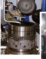
Radial oscillation unit for roller bearing inner rings
